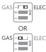
1. When **GAS/ELEC** or **HEATPUMP** is set for **GAS/ELEC**: This switch (**GAS** or **ELEC**) controls how the thermostat will control the Fan (G) terminal in heating mode. When **GAS** is chosen, the thermostat will not energize the Fan (G) terminal in heating. When **ELEC** is chosen the thermostat will energize the fan in heating.
